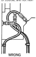
When 90° adapters were used, this assembly became neater-looking and easier to
