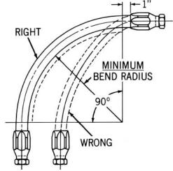
At bends, provide sufficient hose so that it does not have a bend radius less than its recommended minimum bend radius. Too tight a bend may kink the hose and
