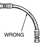
If a hose is installed with a twist in it, operating pressures tend to force it straight. This can loosen the
