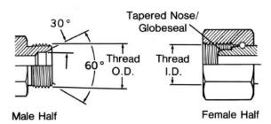
The BSP (parallel) male is similar to the NPSM male except the thread pitches are different in most sizes.
