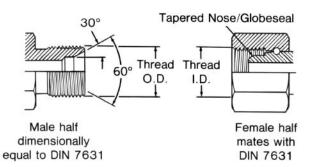
This connection is frequently used in hydraulic systems. The male has a straight metric thread and a 60° (included angle) recessed cone. The female has a straight thread and a tapered nose/Globeseal
