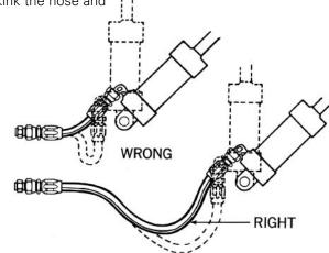
In applications where there is considerable vibration or flexing, allow additional hose length. The metal hose fittings, of course, are not flex-
