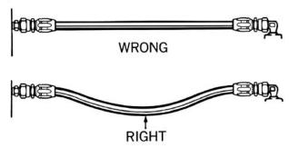
Under pressure, a hose may change in length. Always provide some slack in the hose to allow for this shortening or elongation. (However, excessive slack in hose lines may cause poor appearance.)
