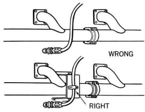
When hose lines pass near an exhaust manifold or other heat source, they should be insulated by a heat resistant boot, firesleeve or a metal baffle. In any application, brackets and clamps keep hoses in place and reduce abrasion. For installations where abrasion to hose cover cannot be prevented with the use of clamps or brackets, a steel protective coil or abrasion resistant sleeve should be placed over the hose.
