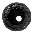
Cause: Indications are that the hose tube is not compatible with the agent being carried. Even though the agent is normally compatible, the addition of heat can be the catalyst that can cause inner liner deterioration. Consult your hose supplier for a compatibility list or present him with a sample of the fluid being conducted by the hose for analysis. Make sure that the operating temperatures both internal and external do not exceed recommendations.
