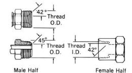
This connection is frequently used in automotive systems. The male connector can either be a 45° flare in the tube fitting form or a 42° seat in the machined adapter form. The
