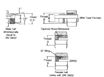
This connection style consists of a common male and three different female halves.
